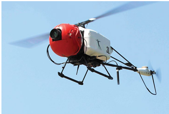
"FieldCopter" used to monitor crop health (AeroVision, sponsor: EC/ Galileo)
